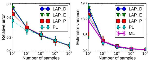
Figure 3. **Left:** Relative error of parameter estimates compared to maximum likelihood for LAP and pseudo-likelihood on a  $4 \times 4 \times 4$  Ising lattice. Error bars show the standard deviation over several runs. **Right:** Variance of the parameter estimates for each algorithm.
