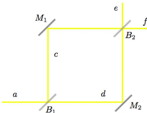
Figure 2.5: A Mach-Zehnder interferometer
