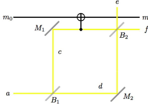
Figure 2.6: A measurement device placed in one arm of the interferometer
