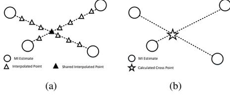
Fig. 6. (a) Loop closure using interpolation method. (b) Loop closure using cross-point method
