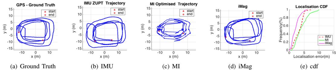
Fig. 10. Experiment 3: Trajectories and CDF for random walking
