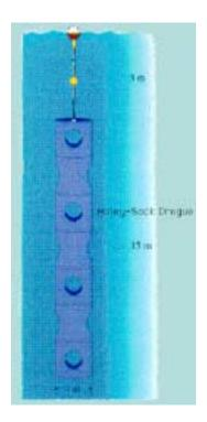
Fig. 1. "holey sock" drifter design
