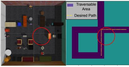
Fig. 4: An example of randomised environments in *ROS Gazebo* and its map. An oracle commander is designed accordingly to give the robot correct commands before it reaches the turning and termination point. The red circle highlights a challenging situation where the intersection is not fully constrained with obstacles which can easily confuse the robot.
