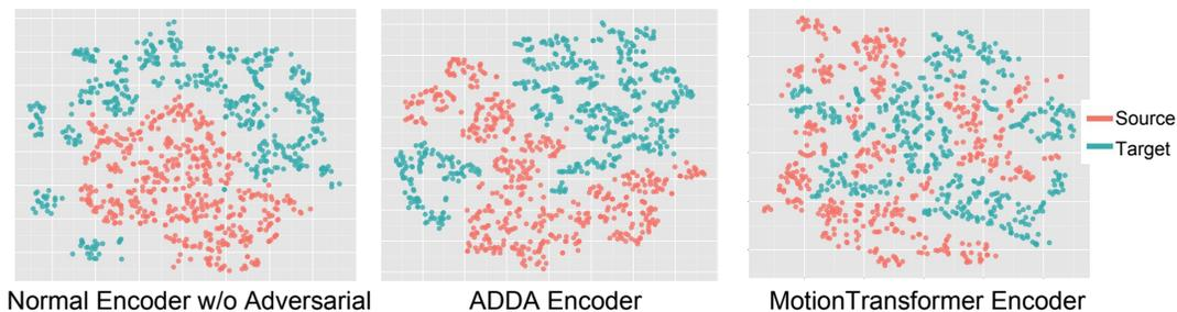
Figure 5: Visualization of extracted representations in the source and target domains. It can be seen that the MotionTransformer leads to a more consistent latent representation compared with the disjoint representations of the normal encoder and the ADDA encoder.
