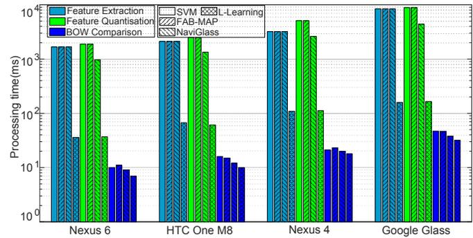
Fig. 15. The running time of feature detection and quantisation per image for different devices. The proposed approach is up to 50× faster than the competing algorithms.
